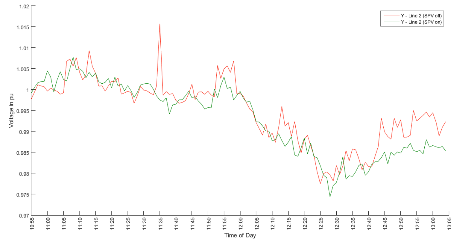
Figure 19: Daily Average Voltage Profile at Maroma for SPV On and Off – Line 2
