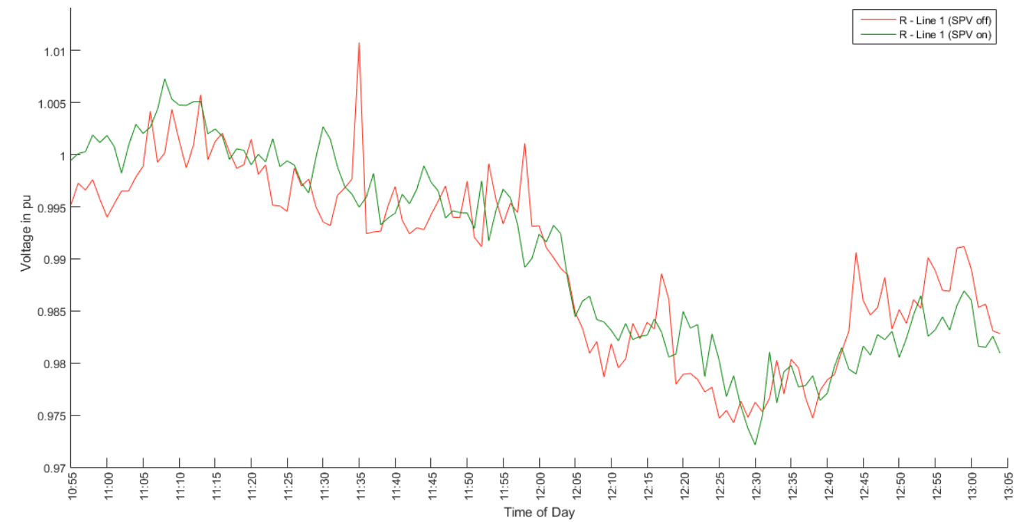
Figure 18: Daily Average Voltage Profile at Maroma for SPV On and Off – Line 1
